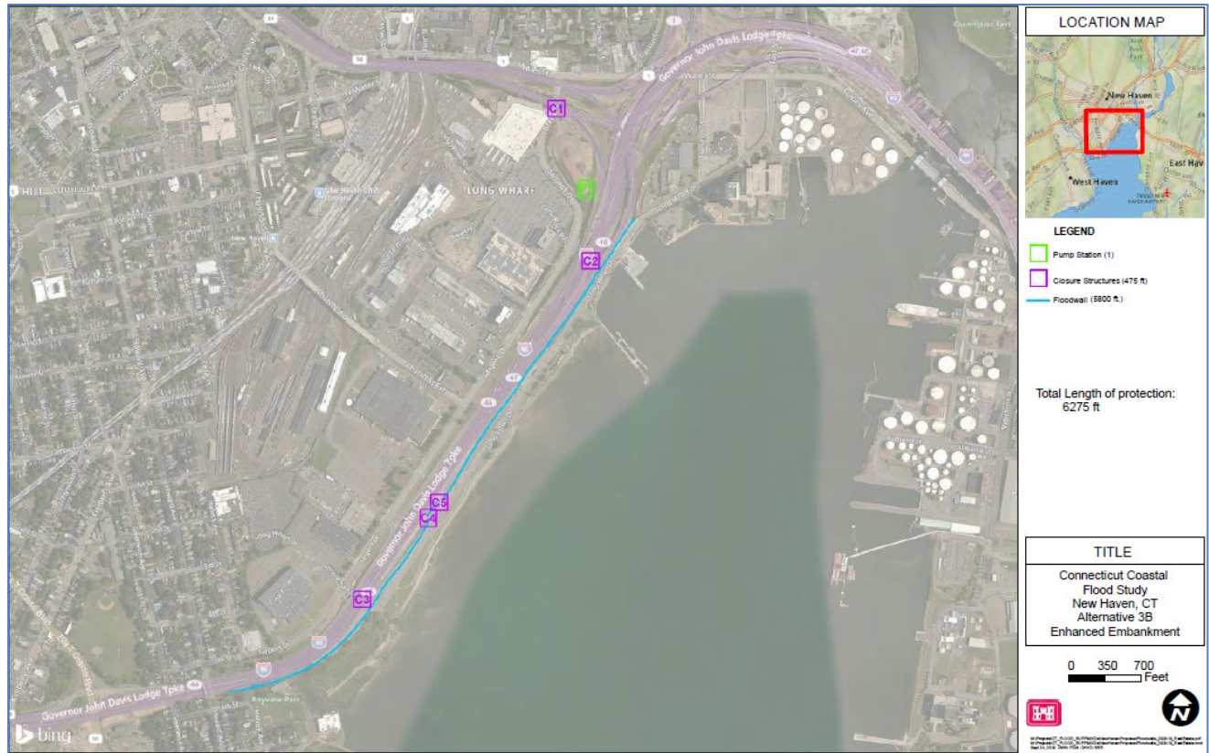
Figure 6 The Recommended Plan, Alternative 3B. The location of the flood wall is shown in blue, closure structures in purple and the 900 CFS pump station is highlighted in green.
